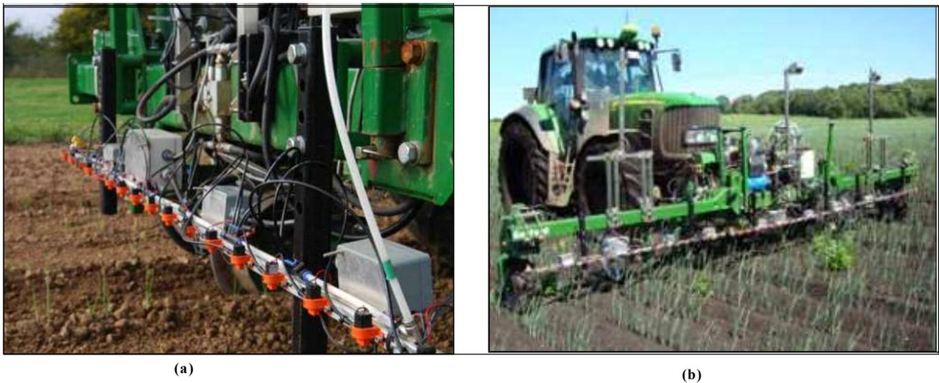
Fig. 3 : (a) The herbicide spot sprayer system (b) Experimental prototype machine
