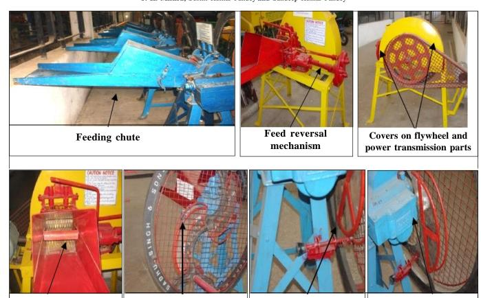
Covers for moving parts: Covers on moving parts that include flywheel, belts, gears, pulleys, feeding rollers, etc. reduce chance of accident during chaff cutting operation. Warning roller: Touch with a wooden roller in feeding chute signals a warning to the operator to pullback his hand to avoid injury from feeding rollers and/or cutting blades.
