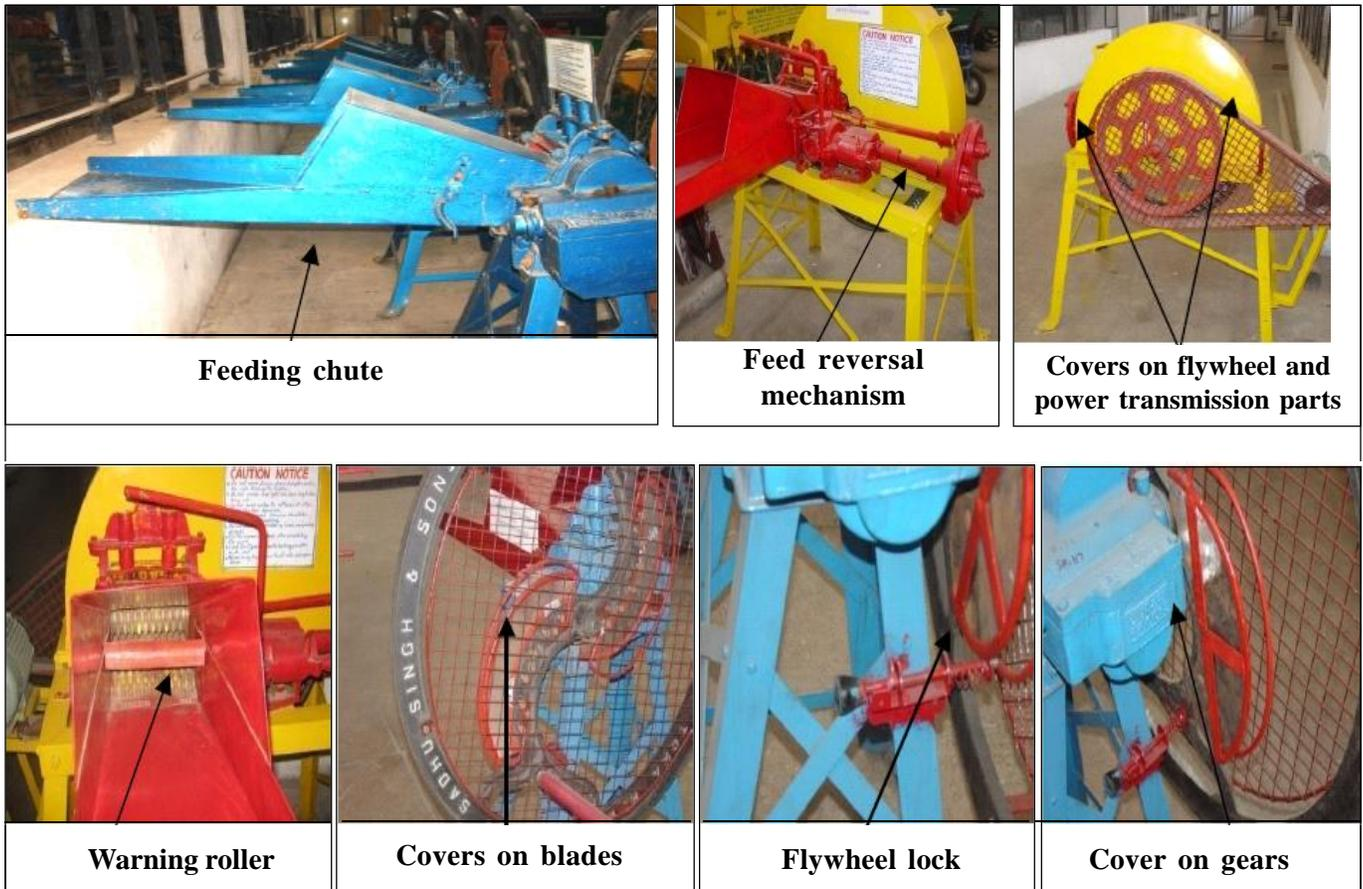
*Covers for moving parts:* Covers on moving parts that include flywheel, belts, gears, pulleys, feeding rollers, etc. reduce chance of accident during chaff cutting operation.
