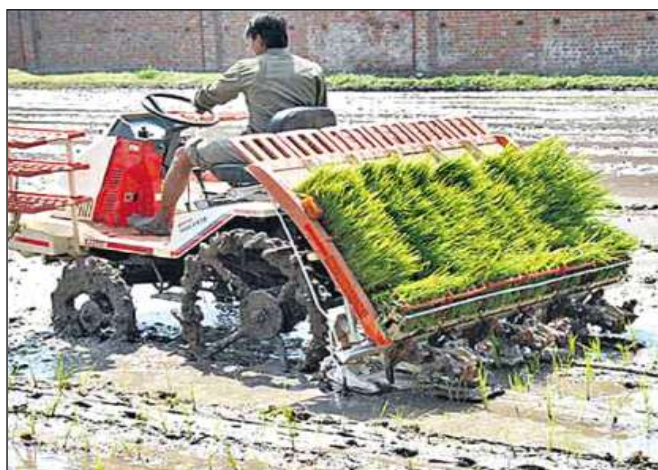
Fig. 1: Self-propelled rice transplanter
