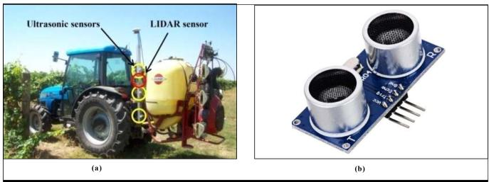
Fig. 2: (a) Sprayer equipped with ultrasonic sensors and LIDAR and (b) Ultrasonic sensor
