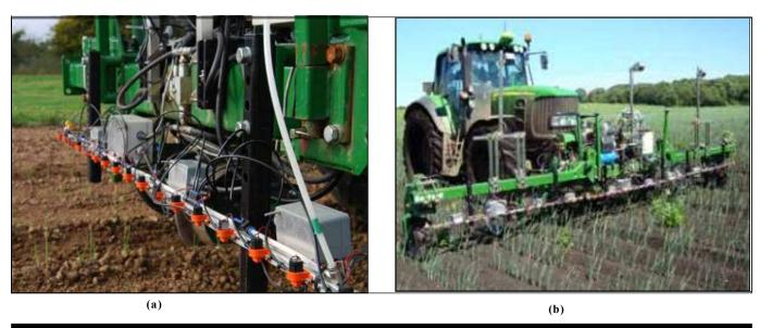
Fig. 3: (a) The herbicide spot sprayer system (b) Exerimental prototype machine
