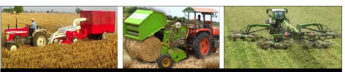
A view of (a) straw reaper combine (b) straw bailer and (c) multi rotor hay rakes for management of paddy and wheat residue
