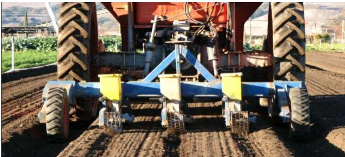
**Cleaning mechanism:** The cleaning mechanism is a new technique which helps to clean the cells of the seed metering device of the planter. It is equipped with the seed metering device. It consists of a spring and a ball.
