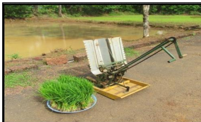
Fig. A : Manual paddy transplanter (hand cranking)
