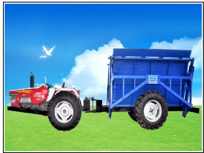
Fig. 4 : A view of sugarcane billets collector and unloader (infielder)
