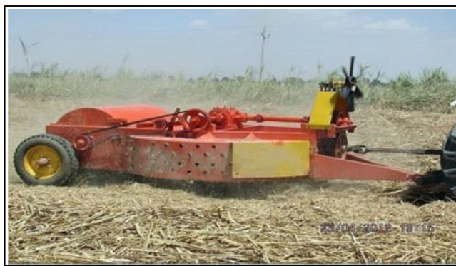
Fig. 5 : Sugarcane trash chopper-cum-spreader machine during field operation
