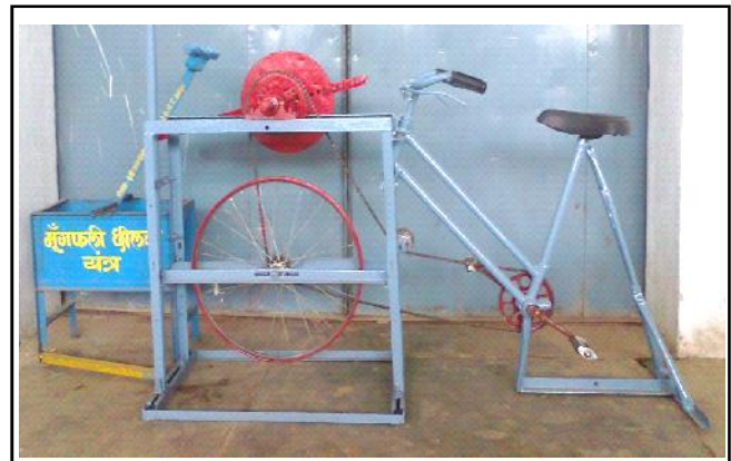
Fig. 3 : Dynapod attached to groundnut decorticator
