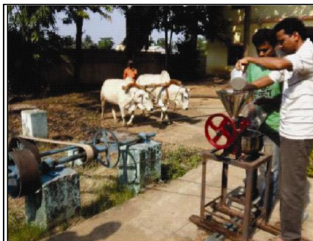
Fig. B : Operation of wet grinder in rotary transmission system using bullocks
