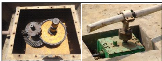
Fig. A : Inside and outside view of Gear box of the rotary transmission system
