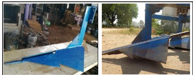
Fig. 1 : Existing iron plough and modified iron plough
