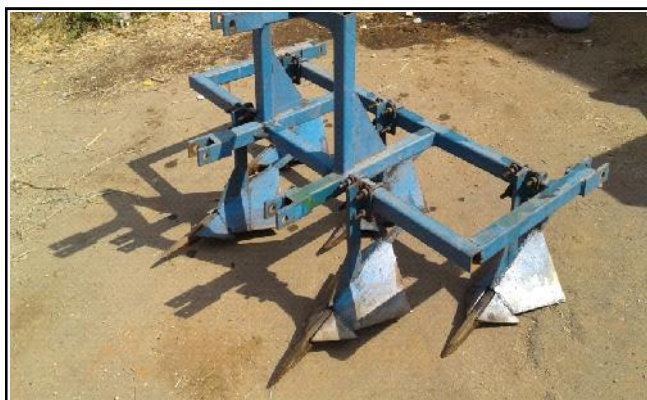
Fig. 2 : Fabricated proto type multi tillage implement with modified iron ploughs
