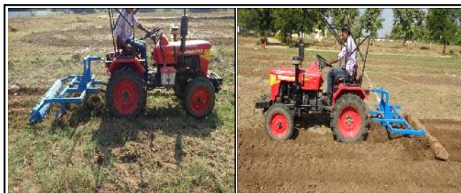
Fig. 3 : Multipurpose tillage implement with clod crusher and planker
