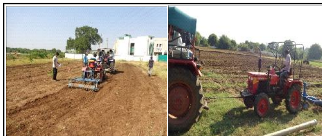
Fig. 4 : Draft measurement of tillage implements
