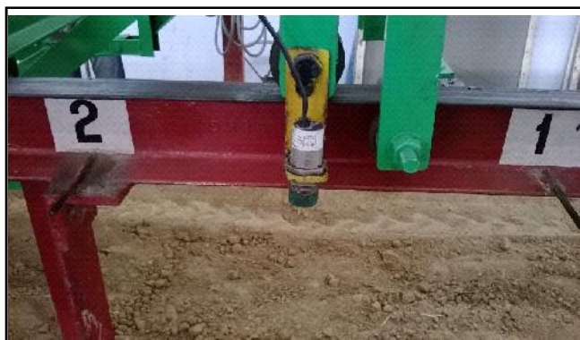
Fig. K : Proximity switch attached on guide trolley for measurement of actual speed
