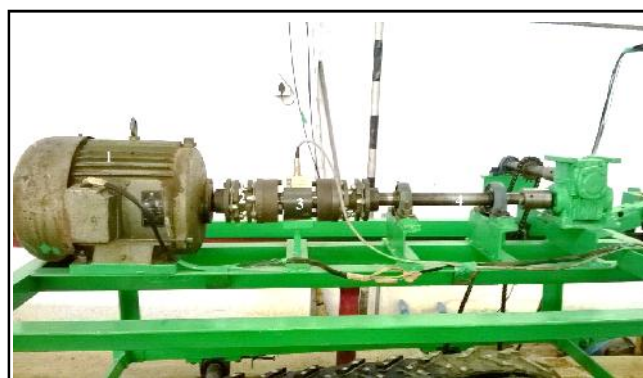
Fig. D : Torque transducer mounted between prime mover and load shaft 1. Induction motor, 2. Bellows coupling, 3. Torque transducer
