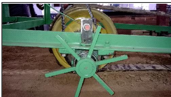
Fig. J : Proximity switch attached on main frame with steel ring with projections on drive shaft for measurement of rpm of drive wheel
