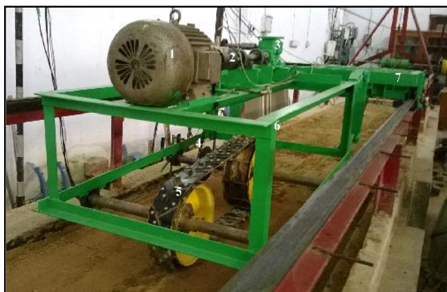
Fig. B : Constructional details of track tester 1. Induction motor 2. Torque transducer 3. Gear box 4. Chain drive 5. Test track 6. Main frame 7. Guide trolley
