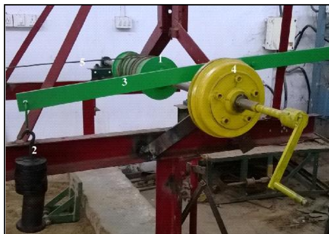
Fig. C : Drawbar loading device 1. Drum 2. Dead weights 3. Lever 4. Shoe type brake 5. Rope
