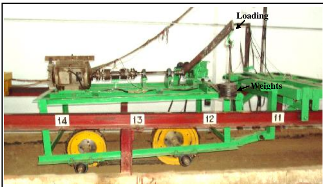
Fig. E : Setup for calibration of torque transducer
