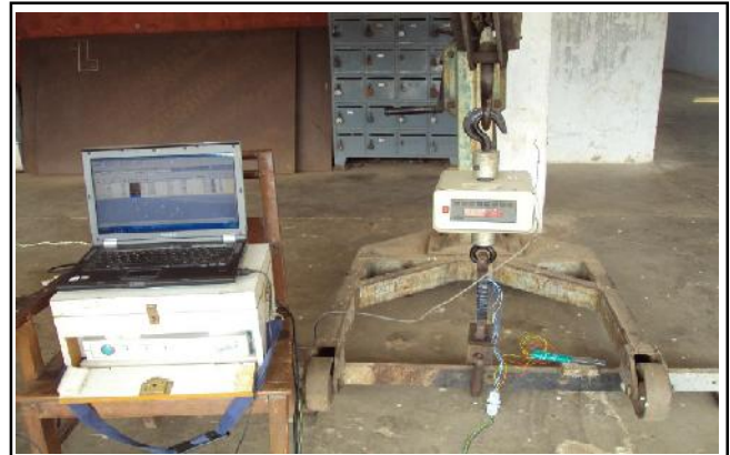
Fig. H : Set-up for calibration of transducer for measuring pull
