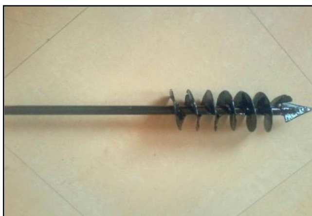
Fig. C : Auger of 100 mm diameter
