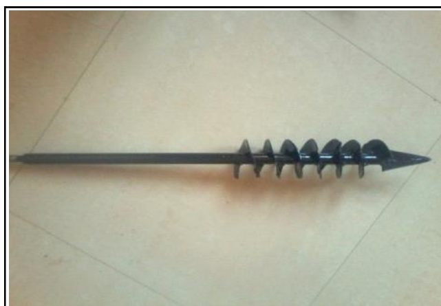
Fig. D : Auger of 70 mm diameter
