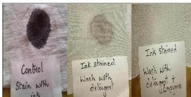
Fig. 12: Washing performance of alkaline protease in the presence of detergent (Tide). (a) Cloth stained with ink; (b) ink-stained cloth washed with detergent only; and (c) ink-stained cloth washed with detergent and enzyme
