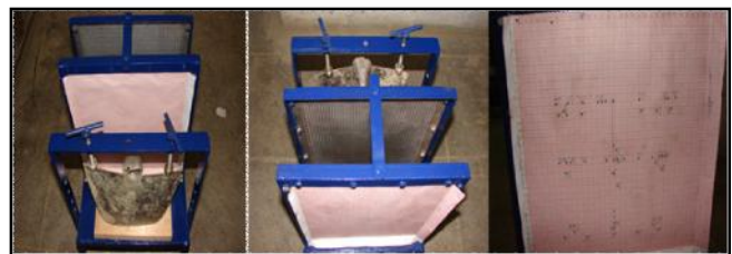
Fig. C: Views of fixture fabricated for measurement of radius of curvature of spade
