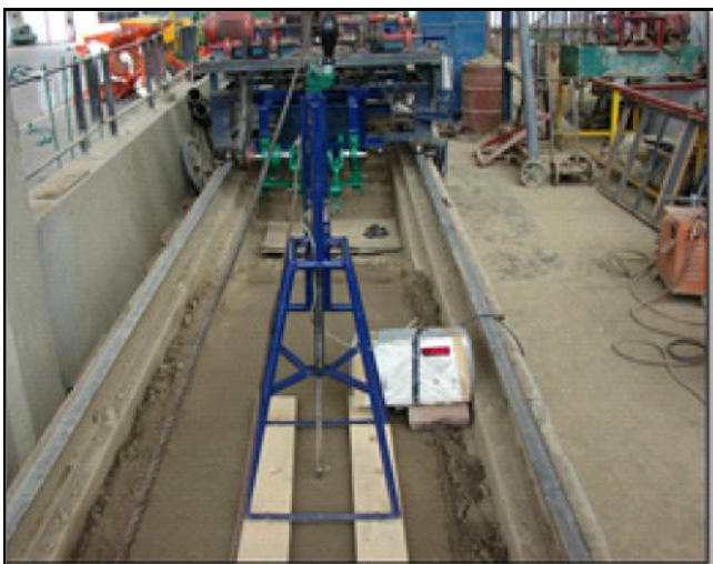
Fig. D: Set-up for measuring cone index in a soil bin
