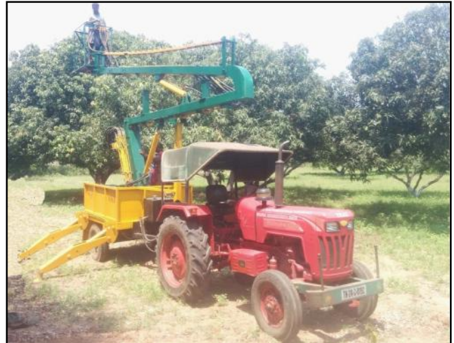
Fig. 1 : View of the developed hydraulic ladder attached to tractor
