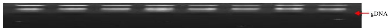
Fig. 1: Bands of genomic DNA extraction using CTAB method, run on 0.8 per cent agarose gel
