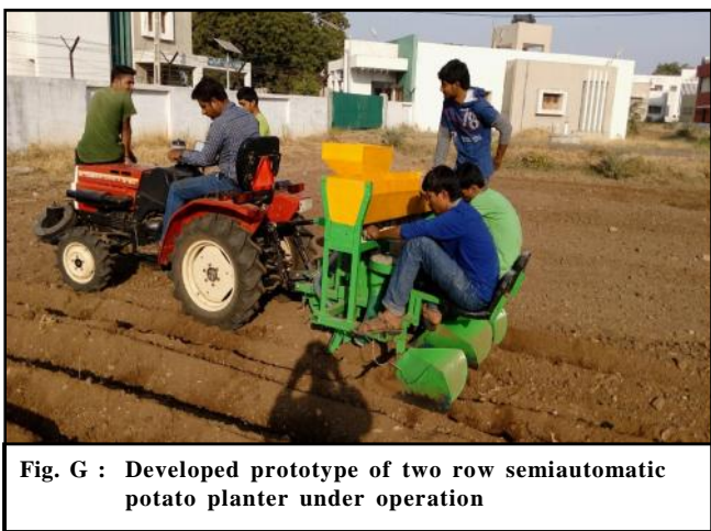
Fig. F : Developed prototype of two row semiautomatic potato planter
