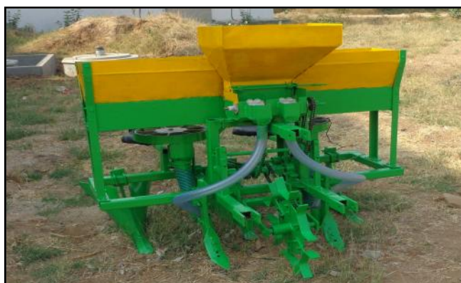
Fig. F : Developed prototype of two row semiautomatic potato planter
