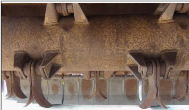
Plate A: Flail blade mounted on center shaft in zig-zag manner
