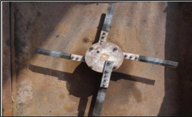
Plate B: Straight blade mounted on disk in straight
