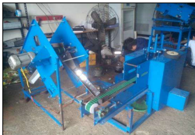
Fig. 3 : Semi automatic chilli stem separator fully fabricated and assembled
