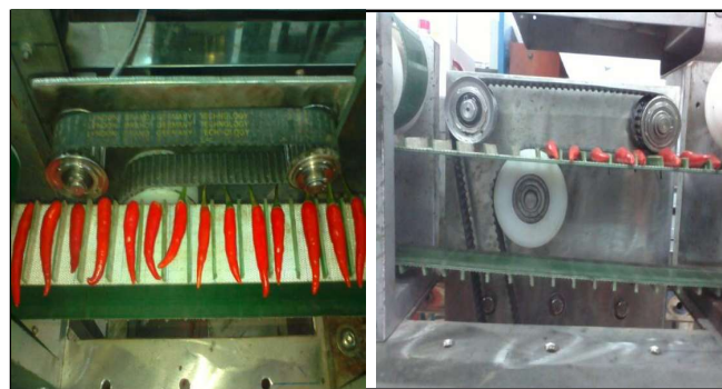
Fig. 4 : Mechanism to separate chilli stalk
