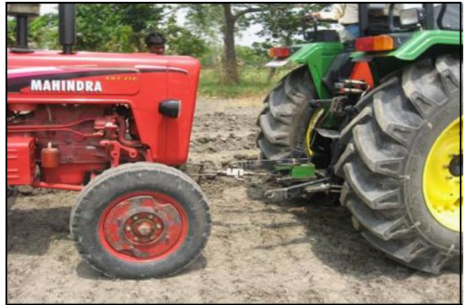
Fig. C : Attachment of S-type digital strain gauge dynamometer for measurement of draft
