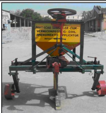
Fig. B: Developed subsoiler-cum-vermicompost and soil amendments applicator
