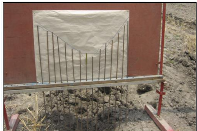
Fig. D : Profilometer for the measurement of soil disturbance by the developed machine
