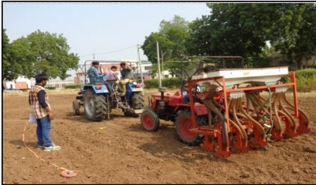
Fig. 10 : Draft measurement of mini tractor with ballasting
