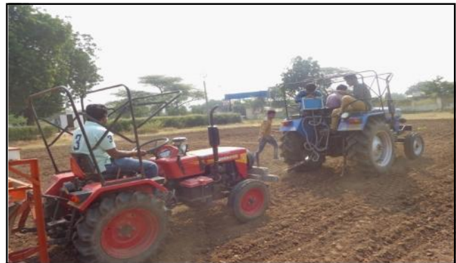
Fig. 7 : Draft measurement of mini tractor with ballasting
