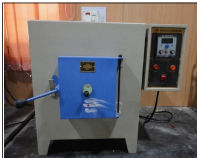
Plate A : A view of hot air oven for determining the moisture content of different biomass material
