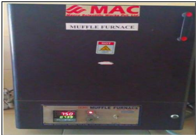
Plate B : A view of muffle furnace for determining the chemical properties of different biomass material
