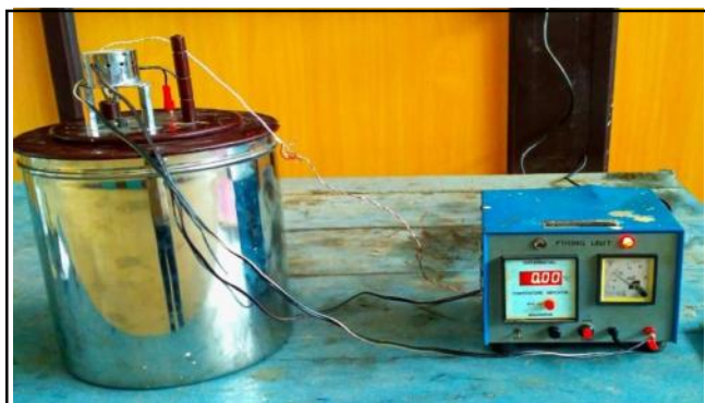
Plate C : A view of bomb calorimeter for determining the calorific value of different biomass material
