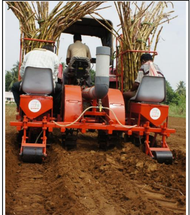
Fig. A : Planting of sugarcane using cutter planter
