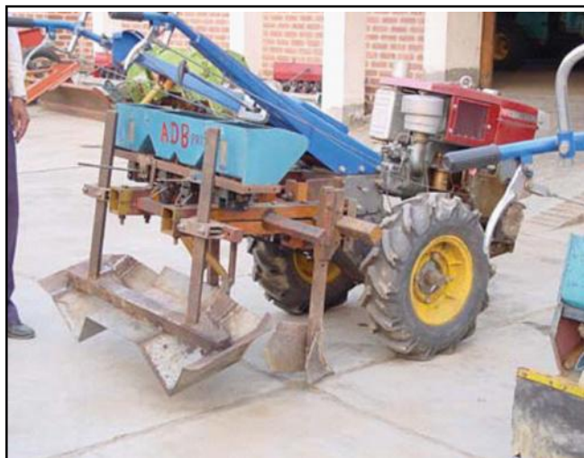
Fig. 4 : Bed planter based on toolbar formers in Bangladesh
