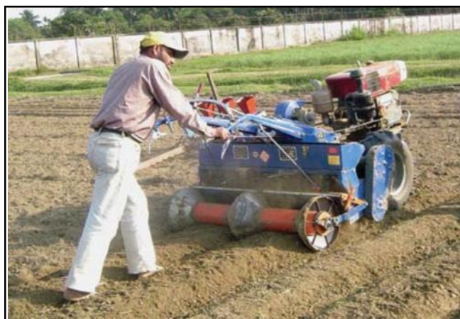
Fig. 5 : Bed former based on POTS with the Chinese hand tractor with square and cone shapers
