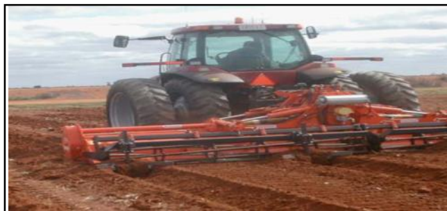
Fig. 8 : Level and smooth seeding surface being created on raised beds by use of a rotary hoe and rotary harrows
