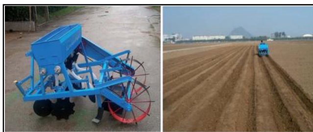
Fig. 6 : Left—the planter for raised bed planting; right - making bed, applying fertilizer and sowing wheat at same time
