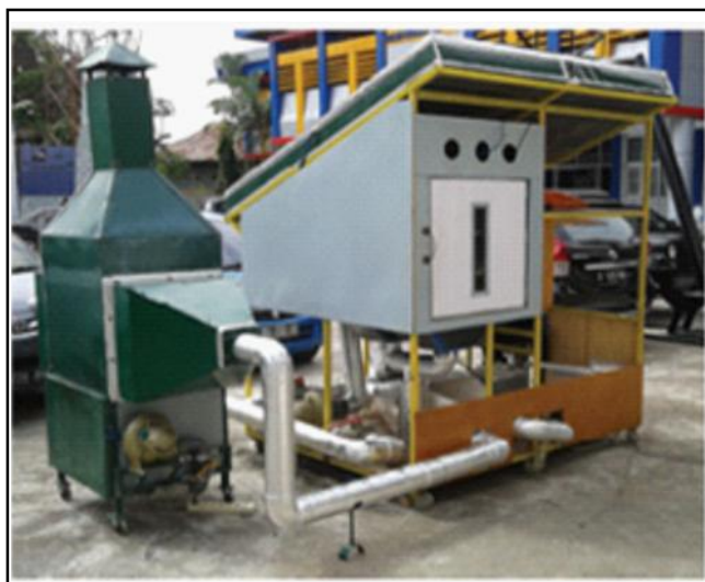
Fig. D : Photograph of solar assisted heat pump dryer integrated with biomass furnace
