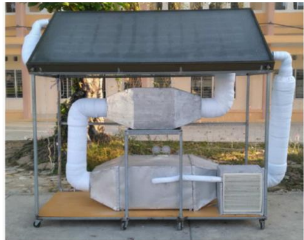
1-Flat plate collector; 2-Drying chamber; 3-Evaporator; 4-Main condenser; 5-Compressor; 6-Secondary condenser; 7-Expansion valve; 8, 9-Exhaust fans; TH1, TH2, TH3, TH4, TH5, TH6- Temperature- humidity sensors
