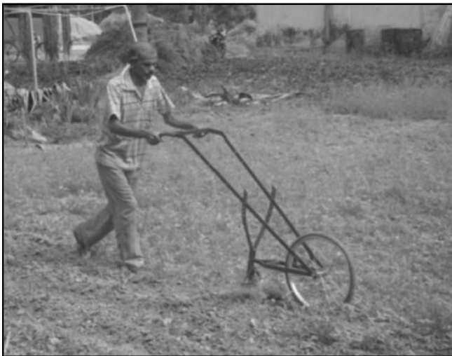
Fig. B: Operation of single wheel weeder
