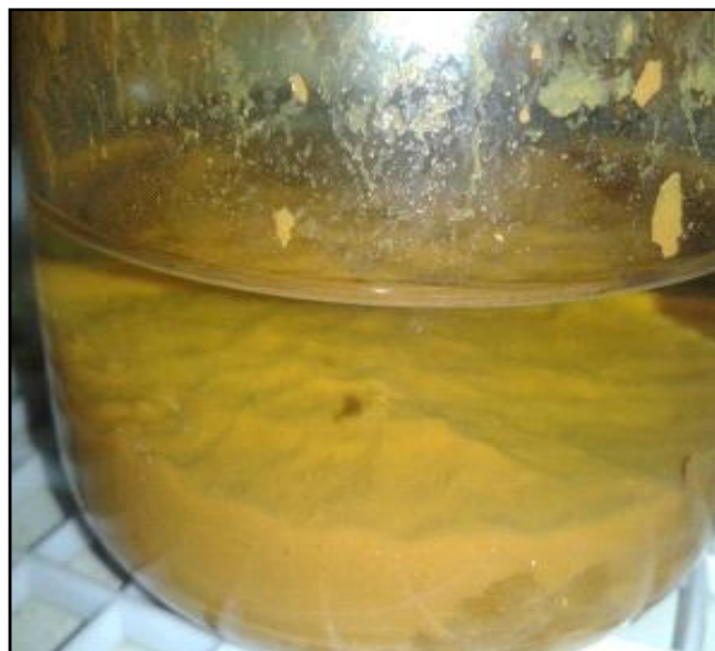
Fig. A : Synthesized crystalline iron-oxide nanoparticle
