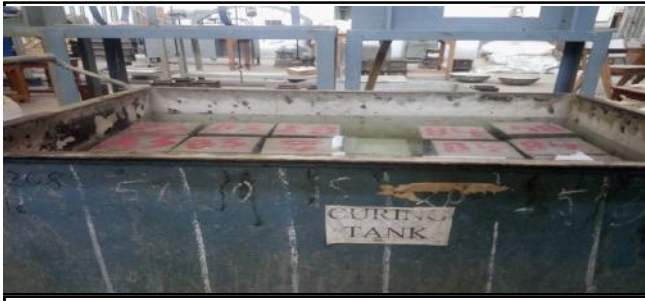
Fig. H : Curing tank
