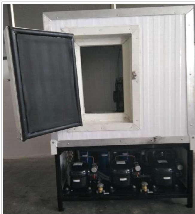
Fig. 1 : Photographic view of nano particle eco friendly chilling plant for fish processing
