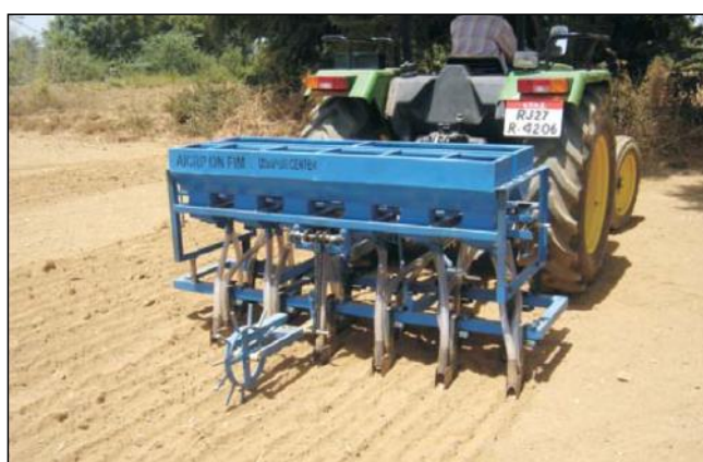
Fig. 7 : Tractor operated MPUAT, Udaipur garlic planter
