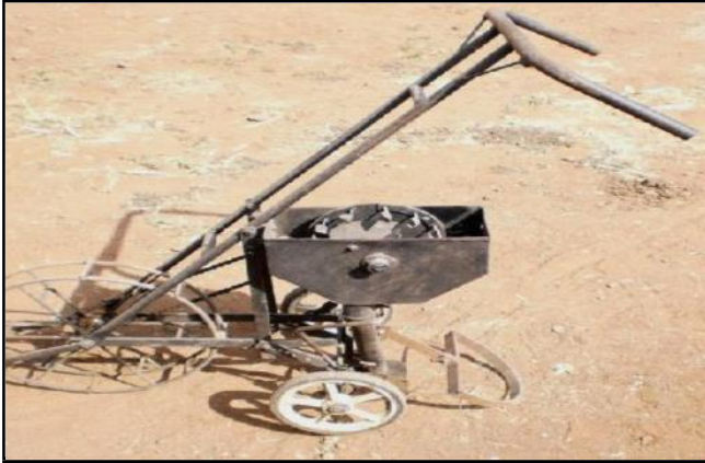
Fig. 3 : Manually operated garlic planter
