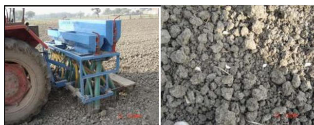
Fig. 8 : Tractor mounted garlic planter in operation
