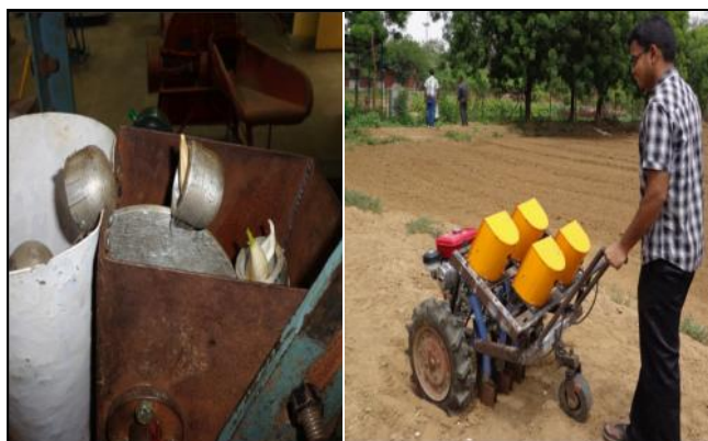
Fig. 6 : Self - propelled garlic planter
