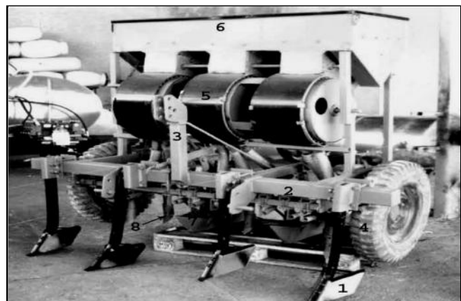
Fig. 11 : Actual picture of the garlic planter (front view): (1) Furrower; (2) Chassis; (3) Three-point hitch mast; (4) Ground-driven wheel; (5) Metering drum, (6) Seed hopper
