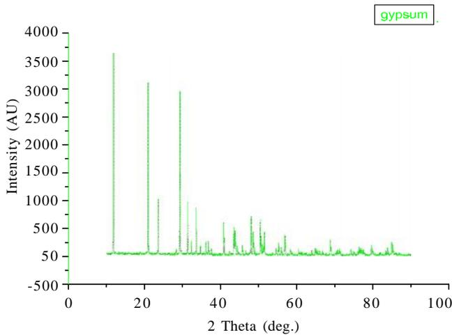
Fig. 1(b): XRD pattern of gypsum
