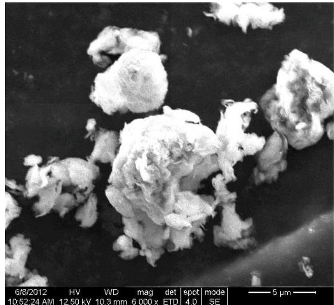
Plate 1(a): SEM image of nano-clay before loading gypsum
