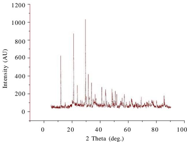
Fig. 1(c): XRD pattern of nano-clay loaded with gypsum
