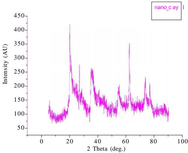
Fig. 1(a): XRD pattern of nano-clay
