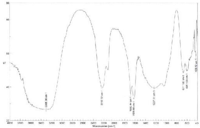
Fig. 3(b): FT-IR spectra of gypsum
