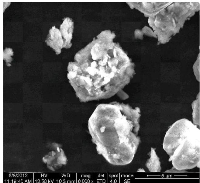
Plate 1(b): SEM image of nano-clay after loading gypsum
