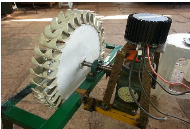
Plate B : Pico-hydro power generation unit
