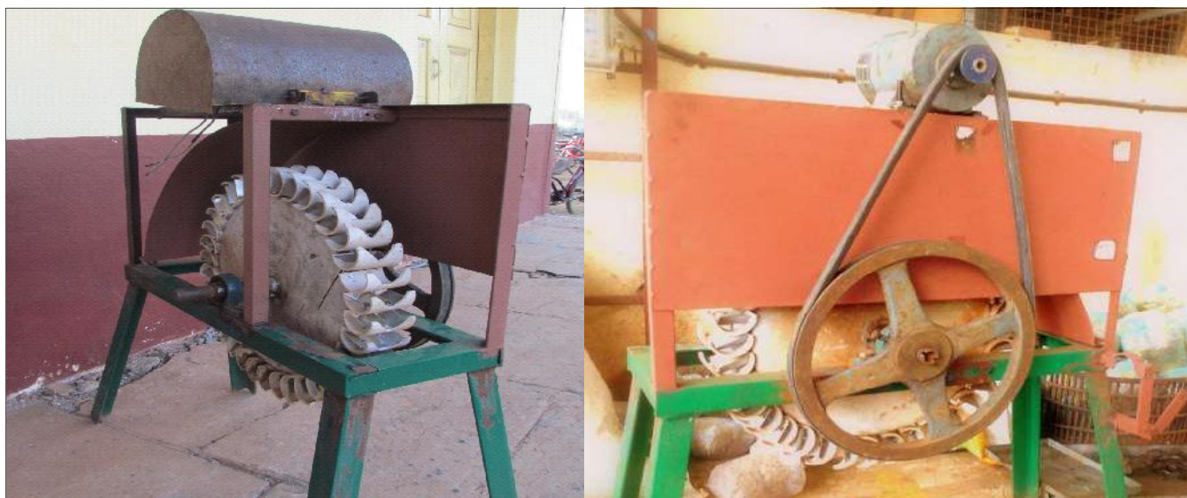
Plate A : Small pico-hydro power generation unit
