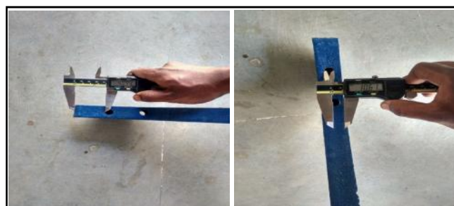
Fig. F&G: Measuring hole center to edge and diameter of the hole of rigid tine using vernier caliper
