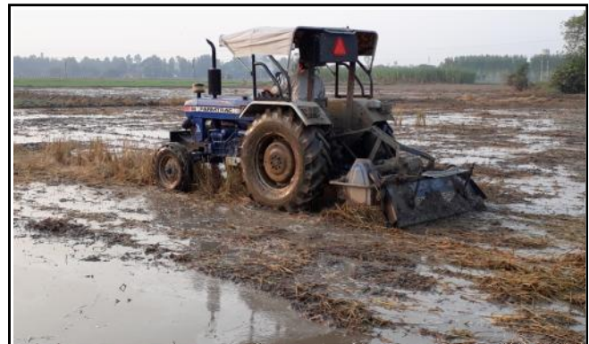
Fig. E : Wet mixing of paddy residue into the soil with rotavator.
