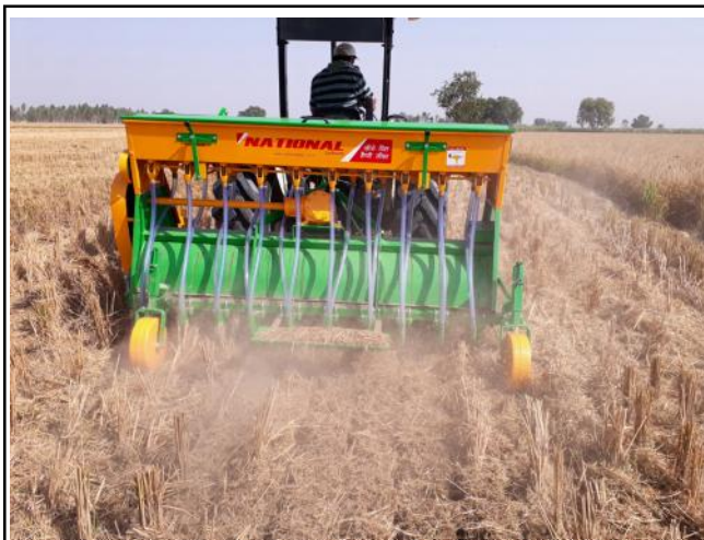
Fig. C : Sowing of wheat with Happy Seeder in paddy residue retention
