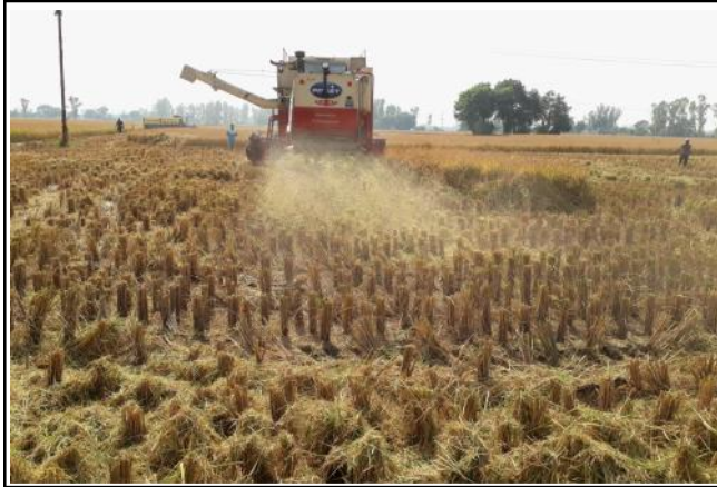
Fig. B : Super SMS attached with Combine harvester in the field
