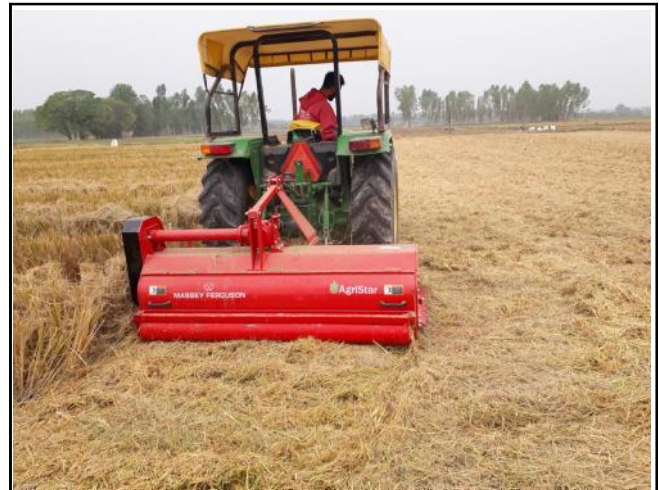
Fig. D : Chopping of paddy residue with mulcher
