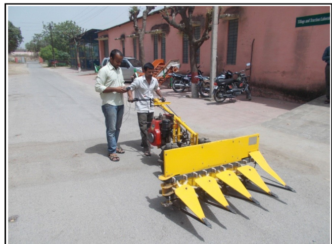
Fig. D : Measurement of HTV of VCR in transportation on bitumen road
