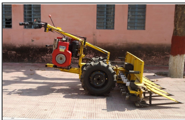
Fig. A : Self propelled vertical conveyor reaper (VCR)
