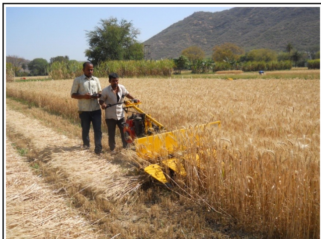
Fig. E : Measurement of HTV of VCR in wheat harvesting operation
