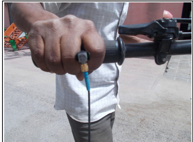
Fig. C : Position of hand on the handle with accelerometer
