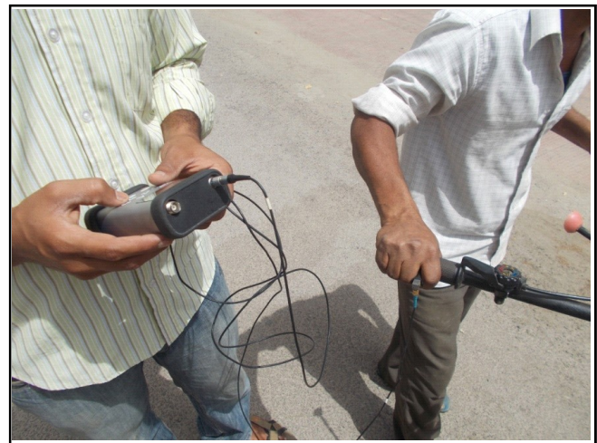
Fig. G : Measurement of vibration magnitudes
