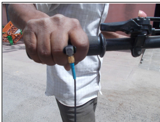
Fig. C : Position of hand on the handle with accelerometer
