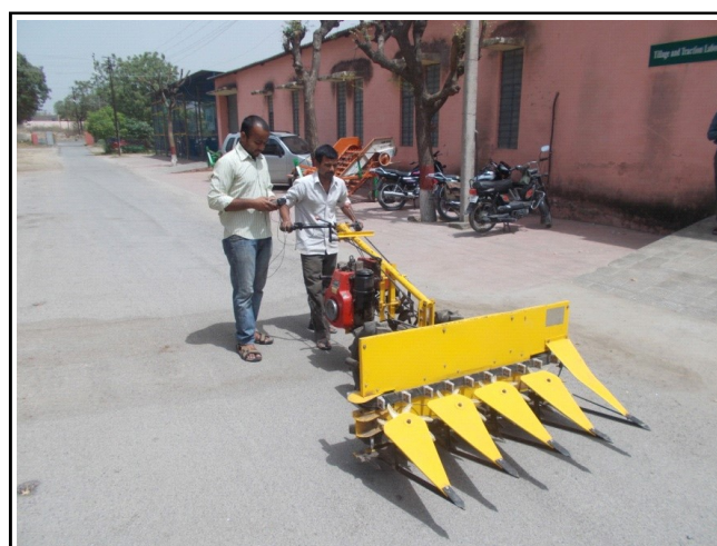
Fig. D : Measurement of HTV of VCR in transportation on bitumen road
