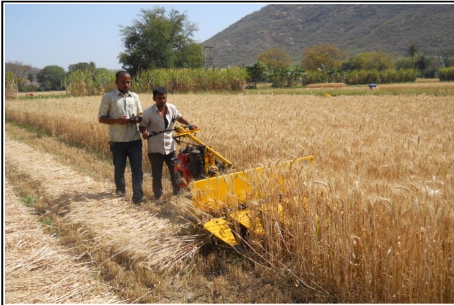
Fig. E : Measurement of HTV of VCR in wheat harvesting operation
