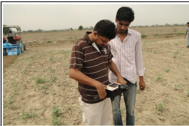
Fig. 3 : A view of digital cone penetrometer to record soil resistance force
