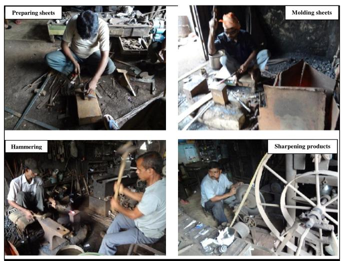
Fig. 1: Workers in odd postures in preparing sheets, molding, hammering and sharpening tools
