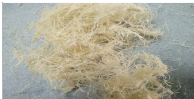
Fig. A : Chemically extracted corn husk fibres
