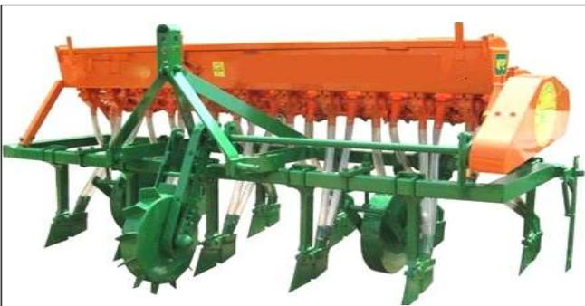
Fig. 1 : Directly sowing of rice by rice planter
