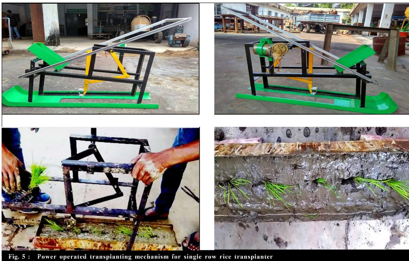
Fig. 5 : Power operated transplanting mechanism for single row rice transplanter
