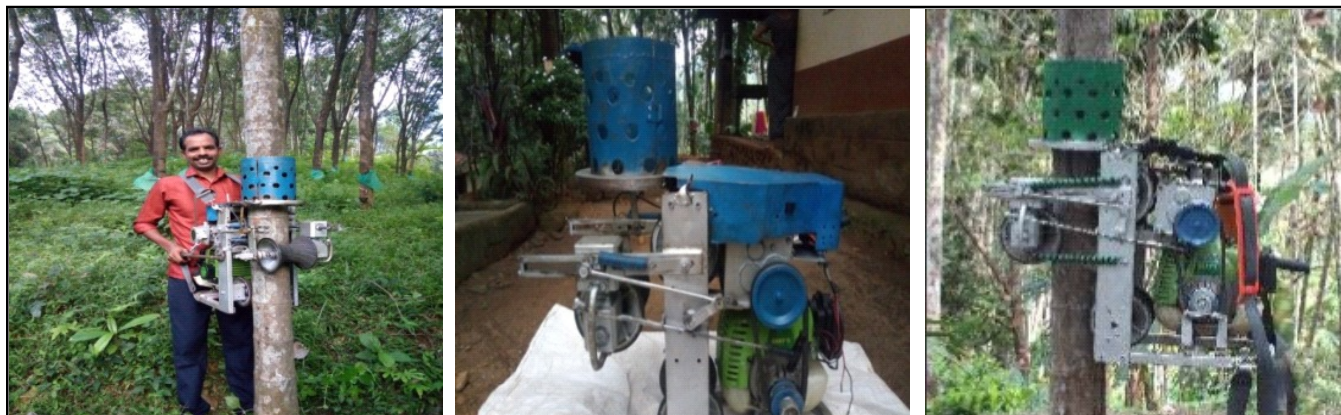
Fig. 3: Automated arecanut climbing and harvesting machine
