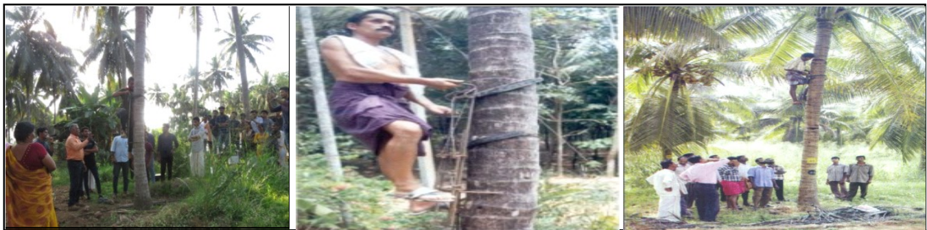
Fig. 1: Tree climber (Device to climb coconut and arecanut)
