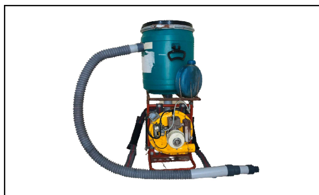
Fig. D: View of knapsack cotton picker with developed picking mechanism and collector
