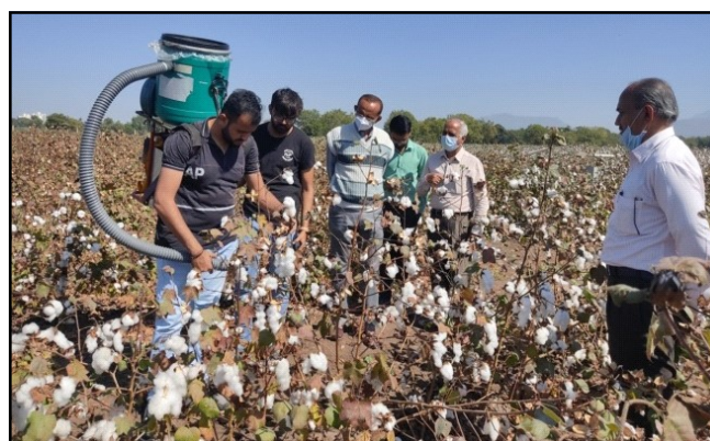
Fig. 3 : Knapsack cotton picker in operation
