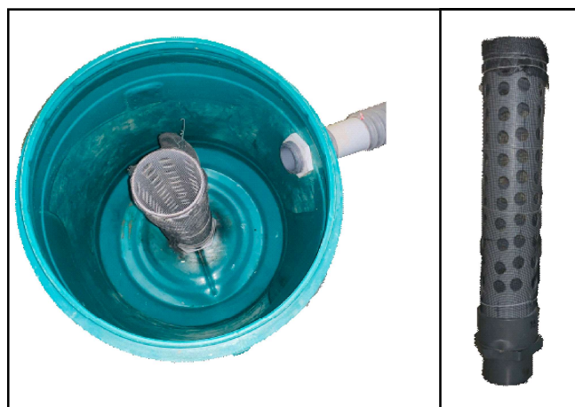
Fig. B : View of collector along with filter
