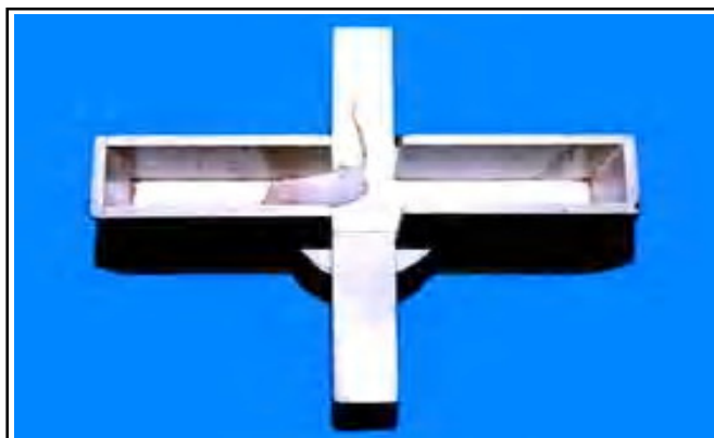
Fig. 1 : Fig.1. Shows elevated plus maze for mice comprising of two open and two closed arms
