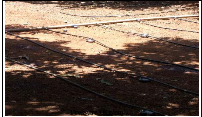
Fig. 1 : Experimental set up for catch cans
