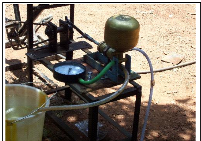
Fig. 2 : Power transmission system for manually operated drip system
