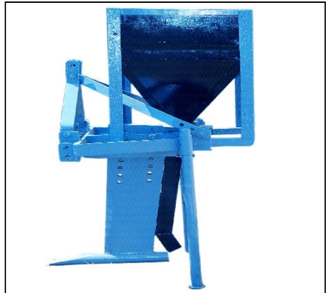
Fig. 2: Newly fabricated mole plough with sand filling system
