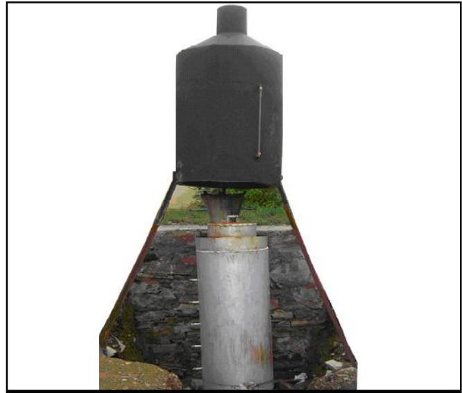
Fig. 2 : Gasifier with heat exchanger system
