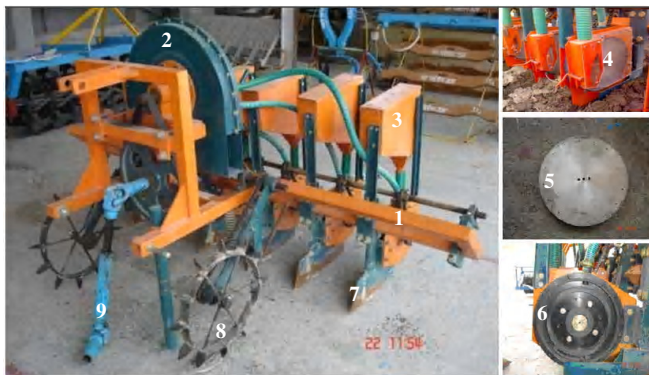
1. Frame 2. Aspirator blower 3. Seed hopper 4. Metering unit 5. Multi groove metering plate 6. Vacuum retaining plate 7. Furrow opener 8. Ground wheel 9. Cordon shaft
